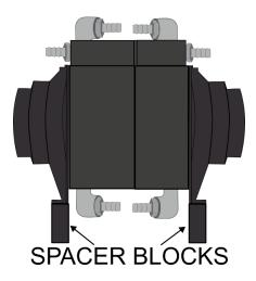
The spacer blocks click into the adaptors and allow a long screw to be fitted down through the block.
