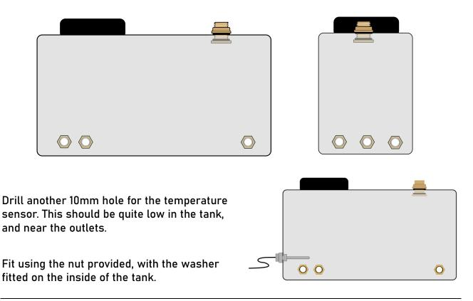
2. BULKHEAD FITTINGS: 4 bulkhead fittings are supplied; the angled outlet is for the overflow and the other three are for the water circulation. Remove the nuts from the smaller brass fittings, apply PTFE tape to the threads and fit as shown
