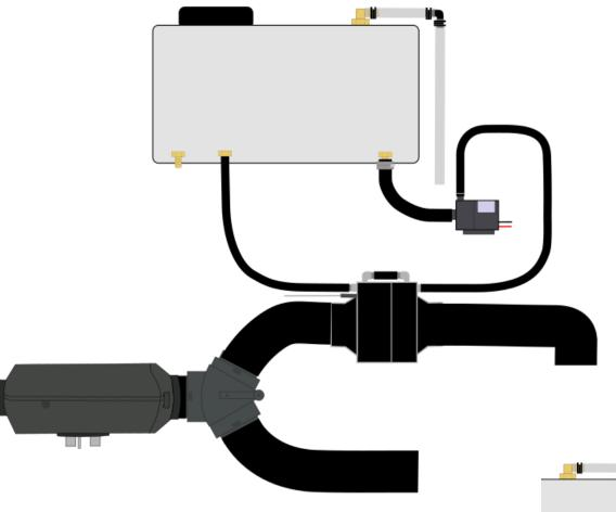
For the overflow pipe, install the PVC pipe to the right angled bulkhead fitting on the top of the tank. This pipe will act as an overflow, so direct somewhere where water can drain safely. The 3<sup>rd</sup> right angled plastic piece can help direct the PVC pipe.
