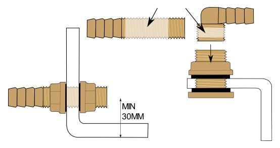
HEAT EXCHANGER ASSEMBLY: Remove the 4 red plastic blanking plugs and 2 metal blanking plugs. Assemble heat exchangers as shown, adding the <u>metal</u> blanking plug into the spare port on the exchanger. Do not overtighten the fittings. Hand tighten only. Add a small piece of the 8mm ID silicone hose to connect the 2 top ports together.
