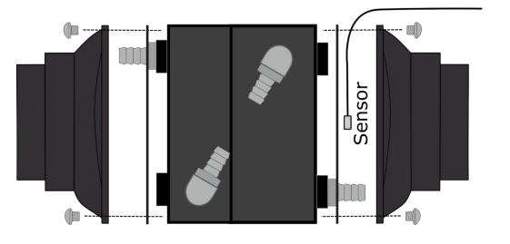
5. DIVERTER ASSEMBLY: Assemble the diverter by clipping together the two halves with the flap in between, then clip on the arm to lock everything together. If you have purchased a remote cable you will also receive a bracket and a small screw. Bend the bracket slightly to get it under the jubilee clip, and install it so that the clip is furthest away from the centre of the diverter as shown.
