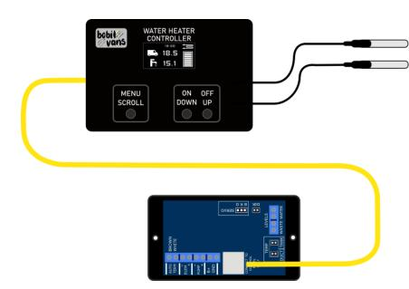
The two boxes are connected via the yellow cable.
