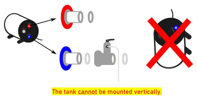
The tank is designed for both barbed fittings or 12mm push fit camper van plumbing. The tank thread is a standard ½" Male thread, for you to screw your needed plumbing adaptors on to.
