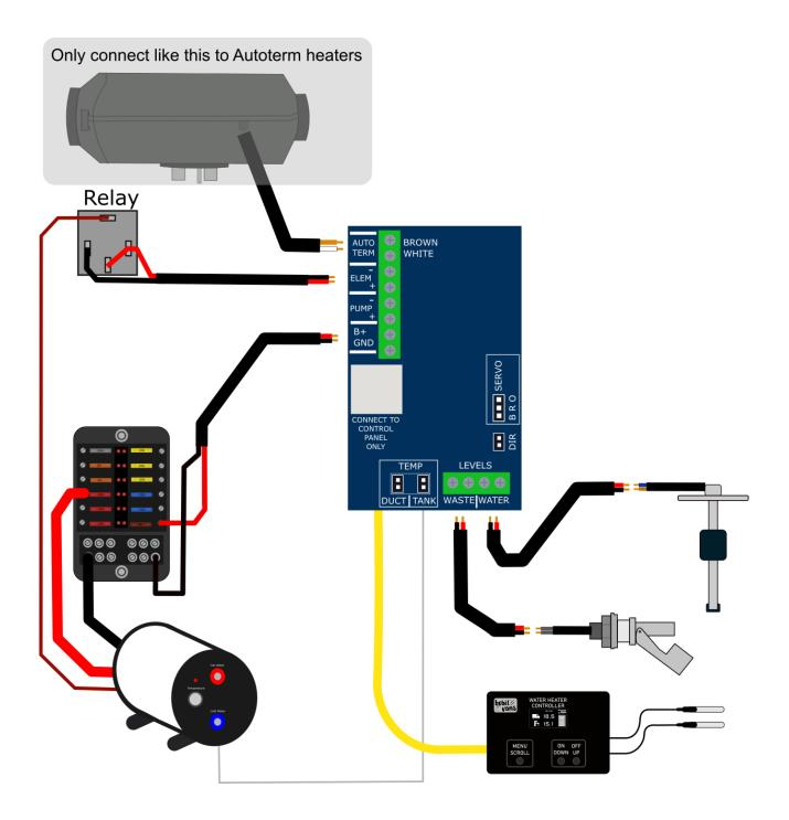
Please note: the "waste" and "water" ports on the bottom right are for the level sensors. If you ordered these, then connect each on to the correct side (there is no polarity). If you did not order level sensors, leave these blank.
