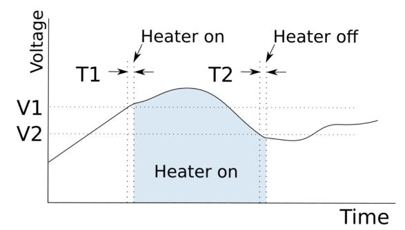
Note that for the element to stay on, you must have enough power coming in to maintain the voltage. If the element is turned on then immediately goes off, it is because the power supplies are not sufficient.
