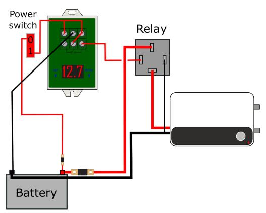
Wire up the controllers as shown above for your tank type. Note that to get an accurate reading the voltage sensitive controller should be wired so that the voltage drop across the cable is no more than 1%.
