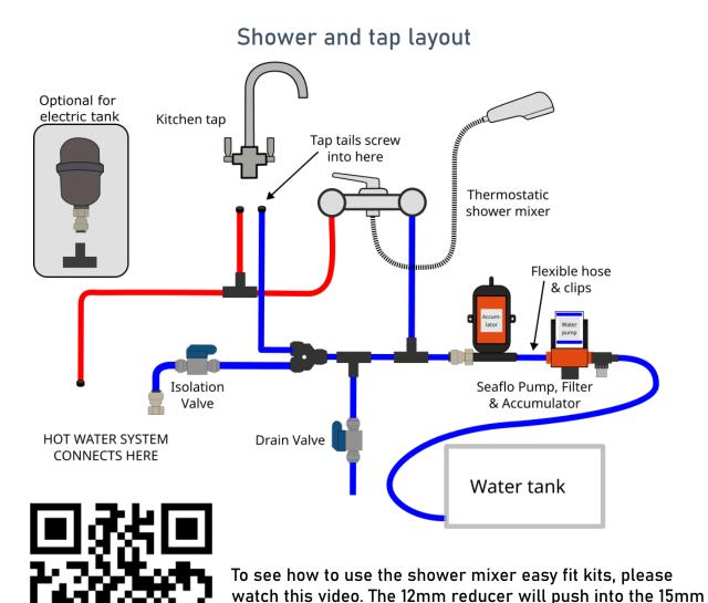
elbow which you can fit on the back of your easy fix kit. To fit the mixer with the pipe inserts, you may need to push the
