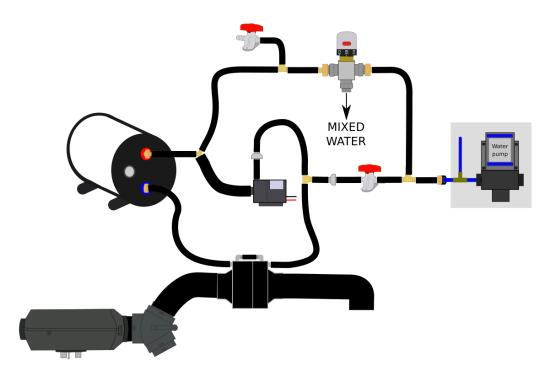
Note- There is an extra drain valve shown at the hot inlet to the thermostatic mixer. This ordinarily remained closed, but if you wish to drain the main tank, then you open this valve. This allows air back into the tank when draining the tank, else there will be an airlock and the tank won't drain properly.
