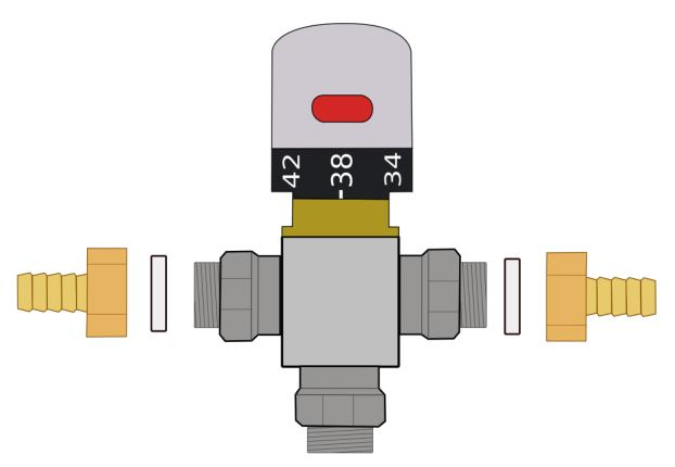
The bottom thread is for your outlet plumbing, so you can screw your fittings directly onto this thread, or you could use a length of hose directly from the barbed fitting. Note that if you want to use a barbed fitting on the output, you should have a spare fitting from the original hybrid kit which can be used here.
